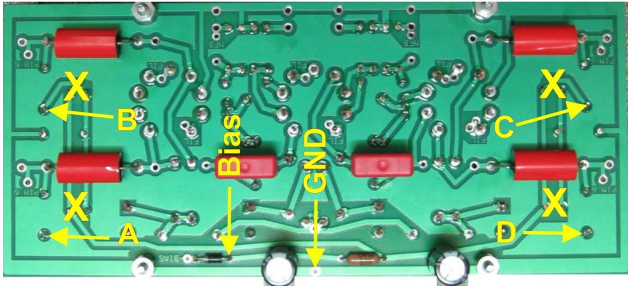
1. Remove the four 10 OHM cathode resistors marked RcatchV2, RcatchV3, RcatchV6 and RcatchV7, connected to pins 1&8 on the four output tube sockets, marked with a **YELLOW X** on the photo
