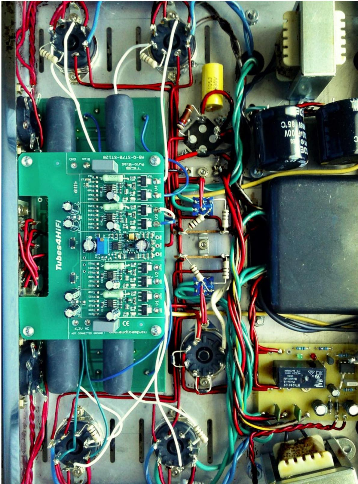
This shows the AB-Q-ST70-ST120 module installed above the ST70/ST120 driver pcb using the supplied spacers and screws and wired up. Keep all of the above wires neat and tidy, maybe use zip ties to group them.
