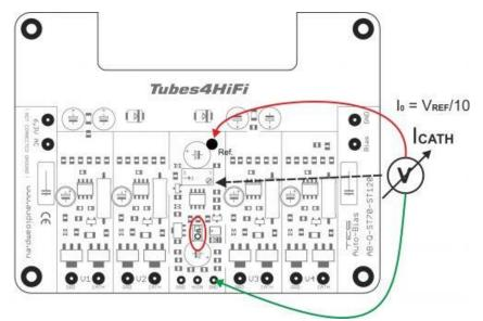
Disconnect the spare transformer or power down your ST70/ST120, wait for half a minute or so and disconnect the wires from the 6,3 AC pads on the AB-Q module.
