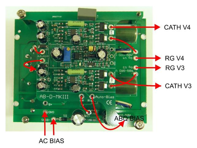
There are no cathode resistors on cathodes V3 and V4. Cathodes V3 and V4 are connected directly to AB-Q-MKIII.
